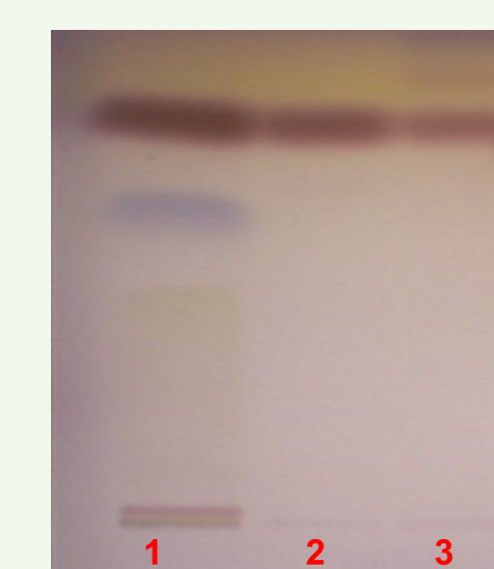
HPTLC plate under white light: 1. Raspberry food supplement; 2-3. Raspberry ketone at 2 different concentrations
