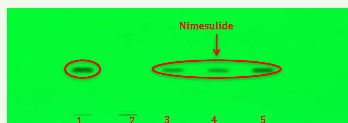
HPTLC plate under UV 254 nm: 1. IPN 2009; 2. IPN 2011; 3-5. Nimesulide at 3 different concentrations
