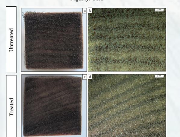
Beech samples inoculated with Aspergillus niger: Application via spray of aqueous solution of CHNPs, CH:Pu 1:0.25 a 0.75 [mg/ml]
